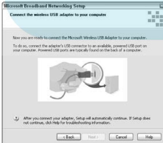
Figure 7-1: Don't connect your wireless network adapter until prompted by the setup software.
